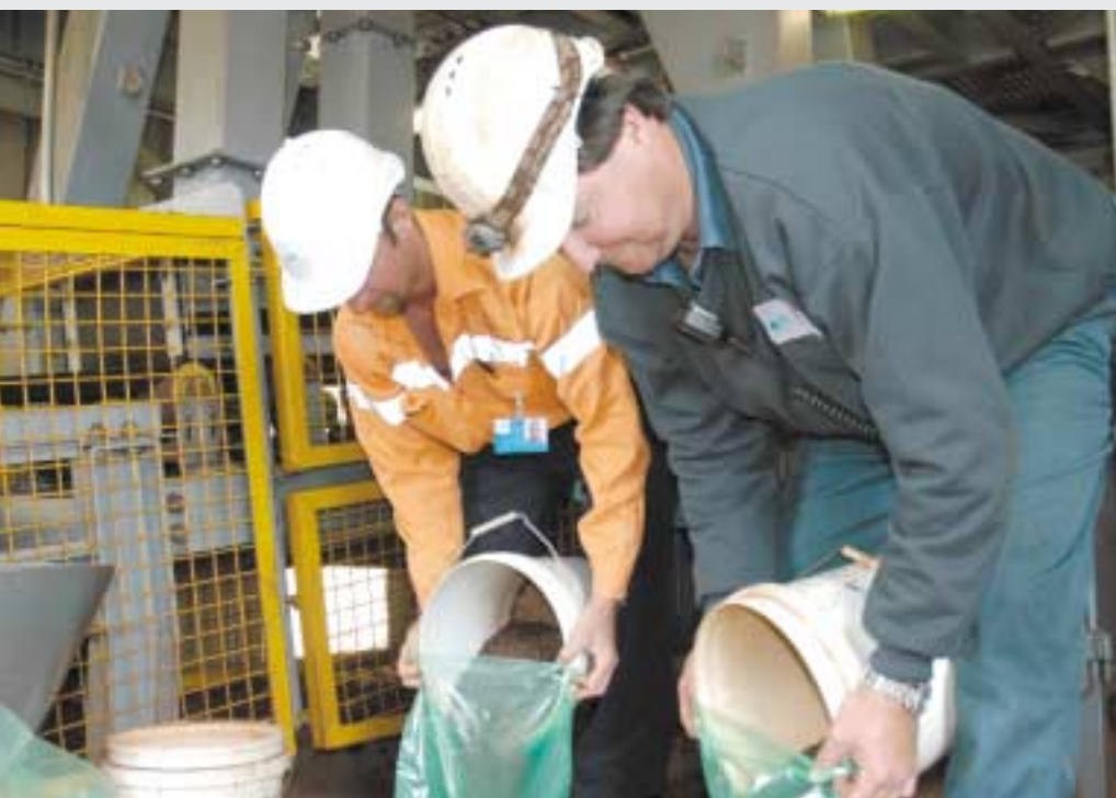
PHOTO TOP: TESTING A DUST SUPPRESSANT ON THE IRON ORE CONVEYOR SYSTEM
